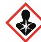
Serious health hazard
